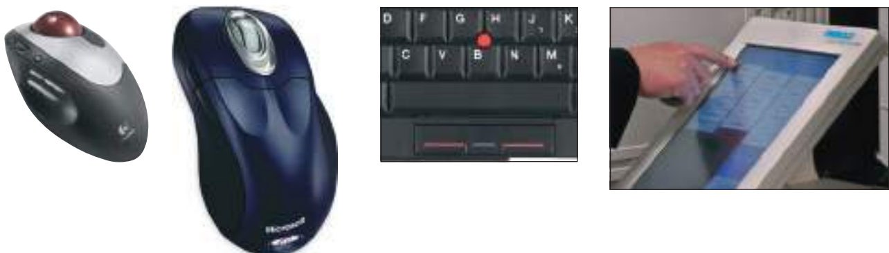
FIGURE 3.15 Many choices exist for pointing devices including the trackball, mouse, pointing stick, and touch screen.
