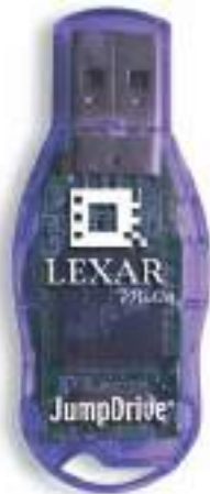
FIGURE 3.26 A USB flash memory drive.
